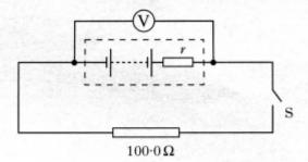
The reading on the voltmeter is  $12.0\,\mathrm{V}$  when switch S is open. The reading drops to  $10.0\,\mathrm{V}$  when switch S is closed.
