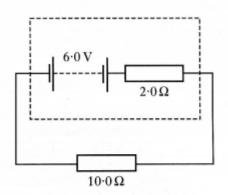
The p.d. across the  $10.0 \Omega$  resistor is
