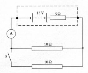
When switch S is closed, the reading on the ammeter changes
